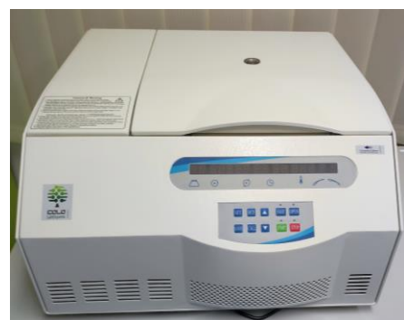
Центрифуга са хлађењем, ВКС-ТН16RШ (swing out rotor for 50 ml tubes;), microtiter plate rotor for 96 well plates; angular rotors for 15 ml and 1.5 ml tube)
